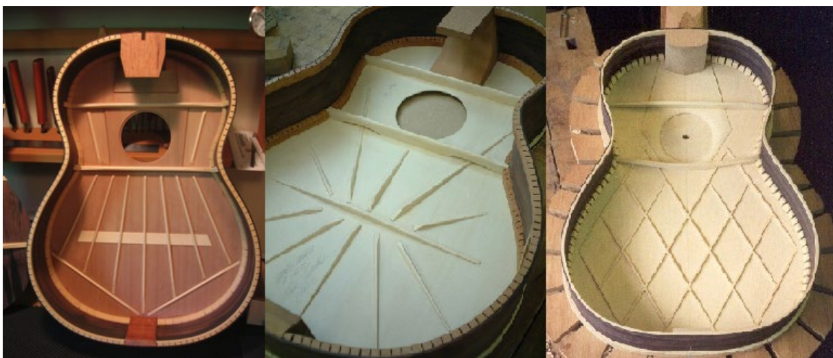
Figure 1. Most popular bracings used in soundboards of guitars [2].
