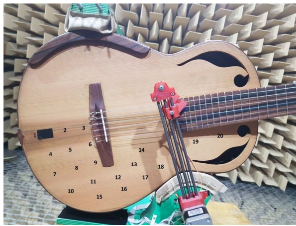
Figure 3. Positions of soundboard vibration velocity measurements.
