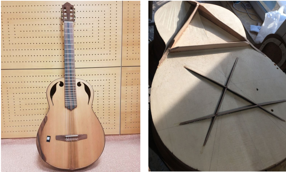
Figure 2. Analyzed guitar with a new shape of the sound holes (left). Variation of the A-bracing used for the soundboard (right).
