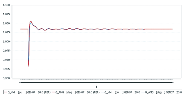
Fig. 4. Generator terminal voltage response obtained for dynamic parameters determined by the genetic algorithm (blue curve) as against benchmark response (red curve)
