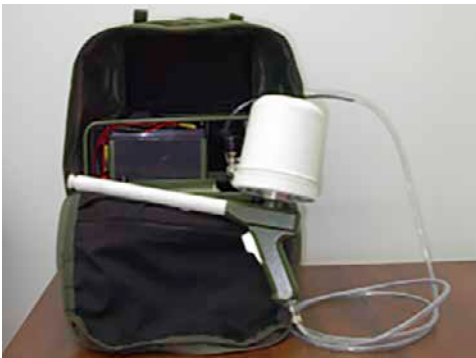
Fig. 14. Autonomous (backpack) device for decontamination with the use of nanosorbents (weight – 9.2 kg, decontamination capability – 10 m 2 of surface) Source: [35].
