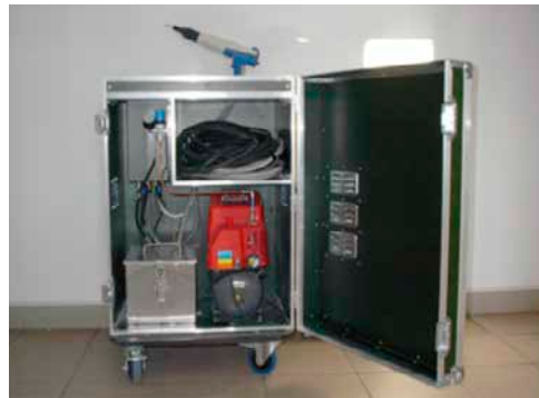
Fig. 15. Mobile device for decontamination using nanosorbents (weight – 63 kg, decontamination capability – 50 m 2 of surface) Source: [35].
