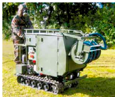
Fig. 5. Decontamination platform – TEP 90 modular system, module 4 Source: [14].
