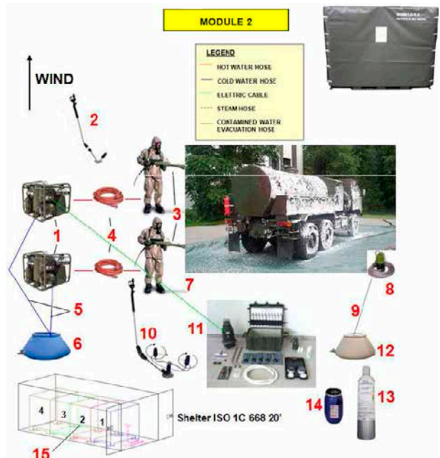
Fig. 9. Variant of the development of equipment decontamination set: 1 – car wash Sanijet C.921, 2 – WW 220M lance, 3 – Sanijet-gun lance, 4 – high-pressure hose, 5 – suction hose of the car wash, 6 – flexible clean-water tank, 7 – water tank after contamination removal, 8 – “dirty” water suction pump, 9 – hose, 10 – chassis washing system, 11 – SX34 CBRN decontamination kit for sensitive equipment, 12 – contaminated water tank, 13 – container for SX34 spray application, 14 – BX24 disinfectant. Capacity: decontamination of 20 vehicles/h (water at the temperature of – 80-85°C and the pressure of 9 MPa) and 20 interiors (vehicle cabins, apparatus, etc.) Source: [15].
