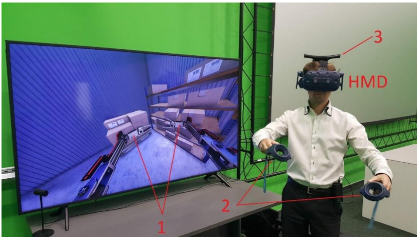
Fig. 2. The image of the virtual environment can be presented in many ways, e.g. on a computer screen or in HMD ( Head Mounted Display ) virtual reality goggles. The illustration shows a training application for operators of a remotely controlled mobile robot with two arms: 1 – operator-controlled virtual robot arms, 2 – controllers used to determine the position and orientation of arms in three-dimensional space, 3 – antenna of the wireless image transmission system to HMD.
