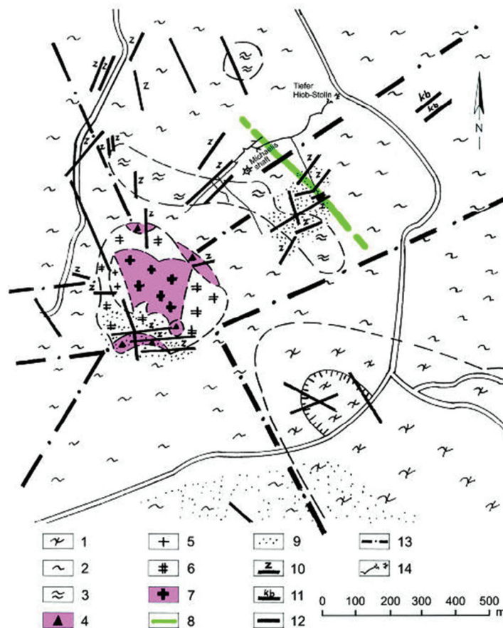
Fig. 5. Geology of the Sn deposit Sachsenhöhe/eastern Erzgebirge (in Seifert 2008, modified according to W. Schilka, pers. comm. 2000, and archive material). 1 – biotite gneiss; 2/3 – muscovite(–biotite) gneiss; 4 – explosive breccia; 5 – syenogranite; 6 – monzogranite; 7 – albite granite; 8 – lamprophyre (type L2); 9 – greisenization; 10 – Sn(-W-Bi) vein-like greisen zone; 11 – “kb ore-type” vein; 12 – vein with post-Variscan mineralization; 13 – fault; 14 – old adit.
