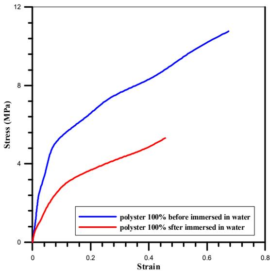
Fig. 11. Stress-strain curve for polyester before and after being immersed in water
