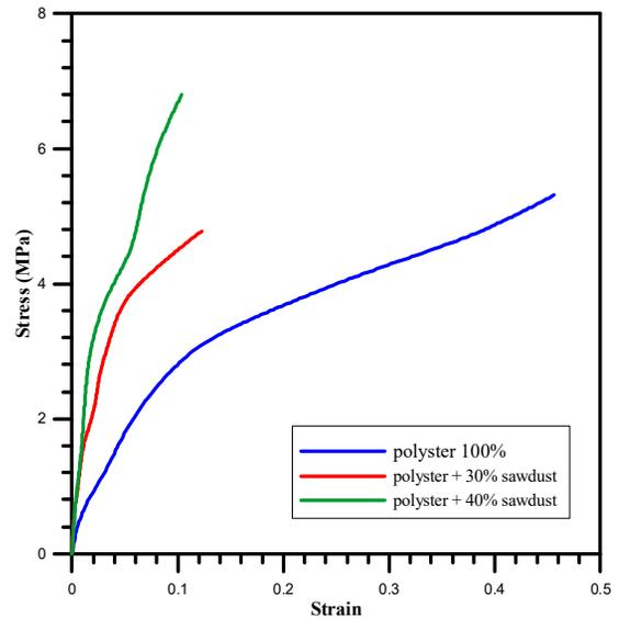
Fig. 10. Stress-strain curve for polyester with sawdust after immersed in water
