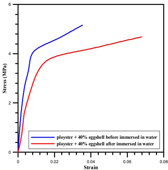
Fig. 15. Stress-strain curve for polyester + 40% eggshell before and after immersion in water
