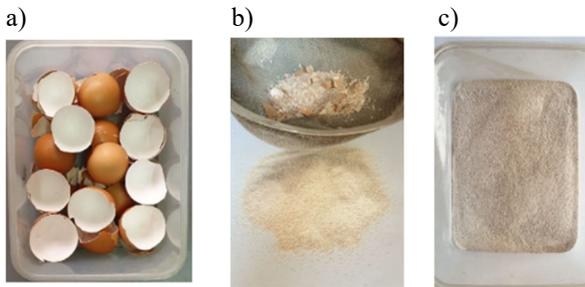
Fig. 2. Eggs shell: a) after cleaning, b) through filtering, c) powder
