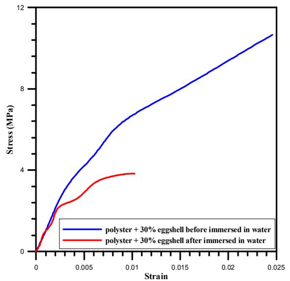
Fig. 14. Stress-strain curve for polyester + 30% eggshell before and after immersed in water
