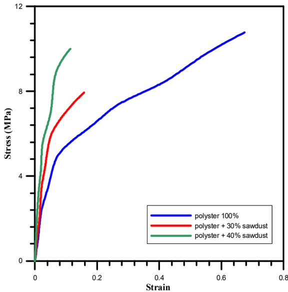
Fig. 8. Stress-strain curve for polyester with sawdust before immersed in water
