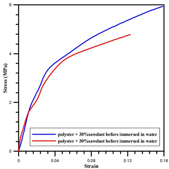
Fig. 12. Stress-strain curve for polyester + 30% sawdust before and after immersion in water
