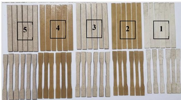
Fig. 5. Bending and tensile samples
