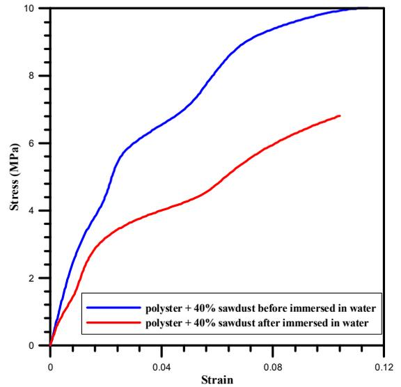
Fig. 13. Stress-strain curve for polyester + 40% sawdust before and after immersion in water
