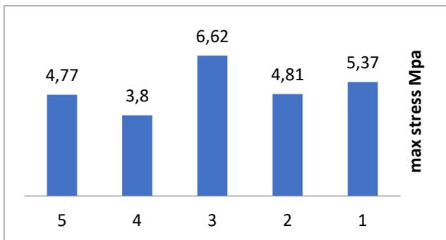
Fig. 17. Maximum bending of stress for a different group of composite materials after immersed in water
