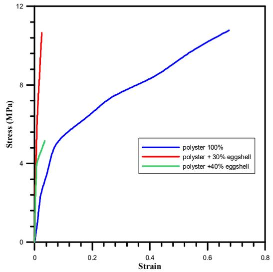
Fig. 9. Stress-strain curve for polyester with eggshell before immersed in water
