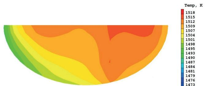
Fig. 5. Temperature distribution in slag cross-section after 150 minutes reduction
