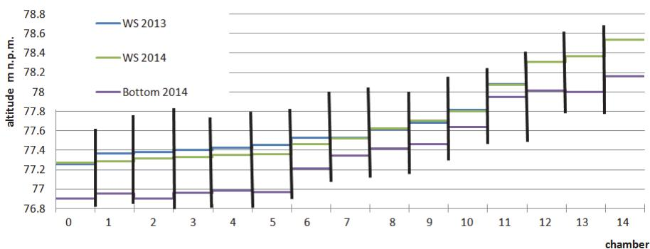
**Fig. 2.** Diagram of the water level topology of the fish pass semi-natural part in 2013 - 2014
