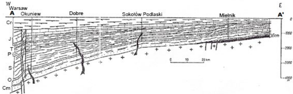
Fig. 5. Geological cross-section along the axis of the Podlasie Depression (Ecm – Eocambrian, Cm – Cambrian, O – Ordovician, S – Silurian, P – Permian, T – Triassic, J – Jurassic, K – Cretaceous, crosses – Pre-Baikal ground, black – Vendian basalt and veins of Paleozoic vulcanites) (Pożaryski 1974)
