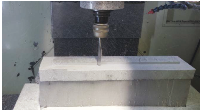
Fig. 7. Start first roughing operation
