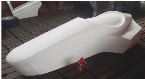
Fig. 4. Model of body used to laminated split fiberglass mold
