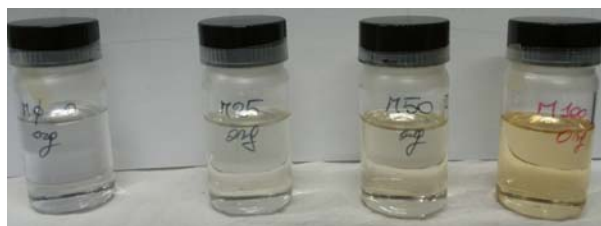
Fig. 1. From the left to the right, mixtures of kerosene + 5 vol.% 1-octanol irradiated to total absorbed dose of 0, 25, 50 and 100 kGy, respectively, and separated from the aqueous phase.
