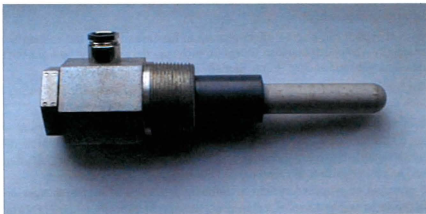
Fig. 2. Platinum plated titanium rod anode (Ti/Pt)
