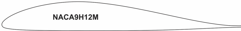
Fig. 4. NACA 9H12M – the reference airfoil for the design of gyroplane-airfoil family [Aut., 2015]
