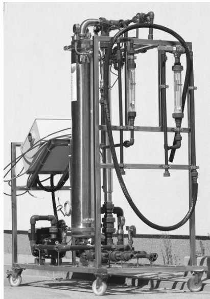
Fig. 2. A general view of membrane microfiltration plant designed to test the regeneration of aqueous operating fluids
