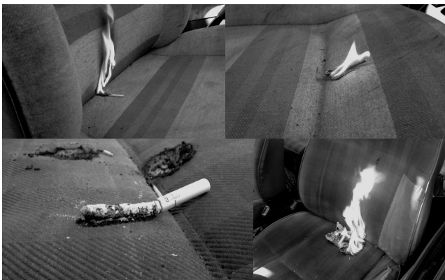
Rys. 1. Sposoby podpalania fotela Fig. 1. Ways of setting the fire to a car seat
