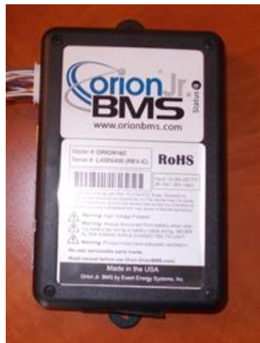
Fig. 5. System BMS ORION
