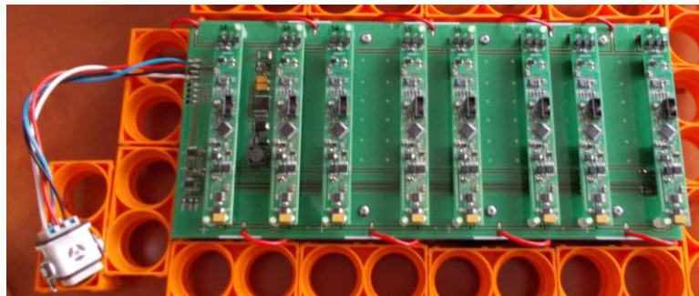
Fig. 7. BMS-S modules installed on the assembly board
