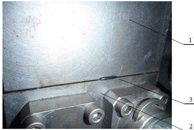
Fig. 7. A view after unsealing the filter 1 – housing, 2 – flow plate, 3 – sealing
