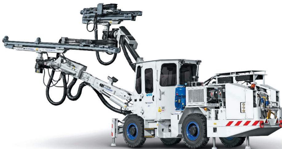
Fig. 3. Face Master 2.3 – two-boom drilling rig
