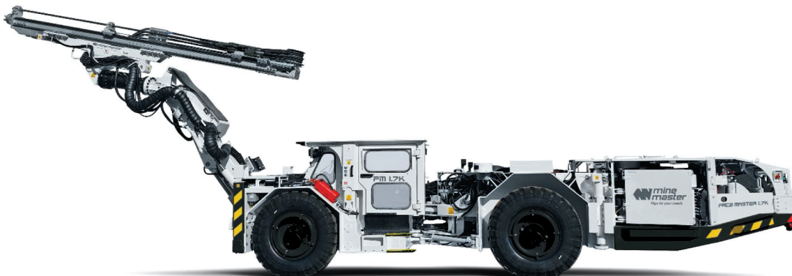
Fig. 2. Face Master 1.7K – drilling rig for low excavations with an air-conditioned cab
