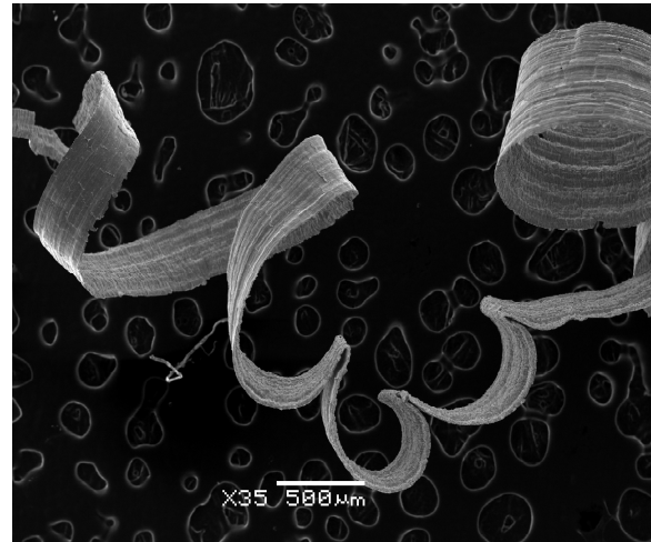
Fig. 7. View of chip for f=0,005\text{mm}\cdot\text{r}^{-1}
