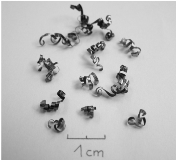
Fig. 2. View of chips for f=0,025\text{mm}\cdot\text{r}^{-1}
