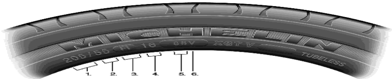
Fig. 3. Tyre construction parameters [8]: 1 – tyre width [mm] = 205 mm, 2 – profile ratio (height to width ratio / aspect ratio) [%] = 55%, 3 – tyre construction – R (radial), 4 – rim diameter code [inches] = 16 inches 5 – maximum load capacity – 88.6 – speed symbol – V
