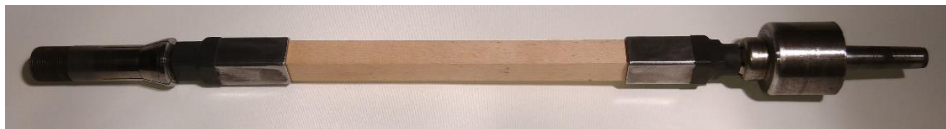
Fig. 4. Mounting of the beam (20 mm × 20 mm) in metal grips and mounts of lathe
