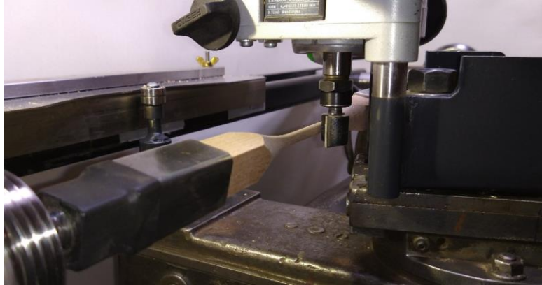
Fig. 5. Mounting of the sample (type F) in lathe and kinematics of machining. The cutting blade of the milling machine is visible in the middle, a piece of lathe spindle on the left side and milling support (in the bottom) coupled with ball-bearing slider moving along metal template (at the top-left side)
