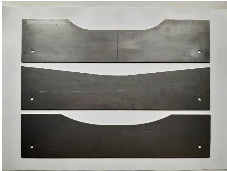
Fig. 6. Stainless steel templates cut out with use of laser and CNC machine, that helped in preparation of samples for tension strength testing (from the top): standard type S, cylindrical with conical tapering type K, cylindrical with funnel tapering type F
