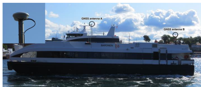
Figure 6. Baronen vessel including location of GNSS antennas
