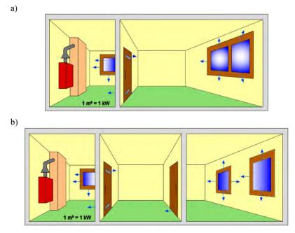
Fig. 3. The appliance is located in directly ventilated room:a) a connection with an adjacent room of the same user,b) a connection through indirect ventilated room of the same user
