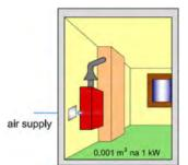
Fig. 5. Location of the appliance of type B with atmospheric burner and draught diverter in cabinet or in separate room with permanent air supply from outside
