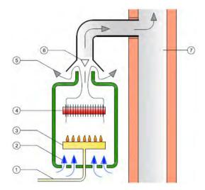
Fig. 2. Gas appliance of type B (water cooker): 1 - gas supply, 2 - combustion air,
