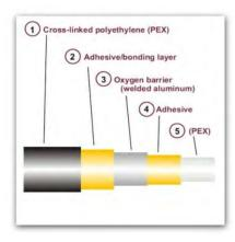
Fig. 11. Scheme for construction of multilayer pipeline ALPEX [8]
