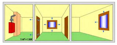
Fig. 4. The appliance is located in indirect ventilated room
