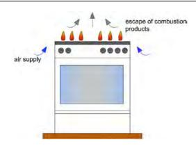
Fig. 1. Gas appliance of type A (cooker)
