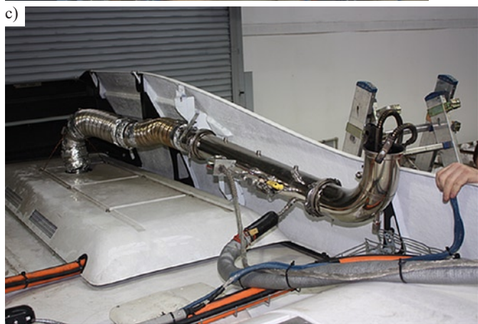
Fig. 3. View of the PEMS equipment during operation on a bus: a) AVL MSS 483, b) SEMTECH DS, c) mass flow meter of the exhaust gas
