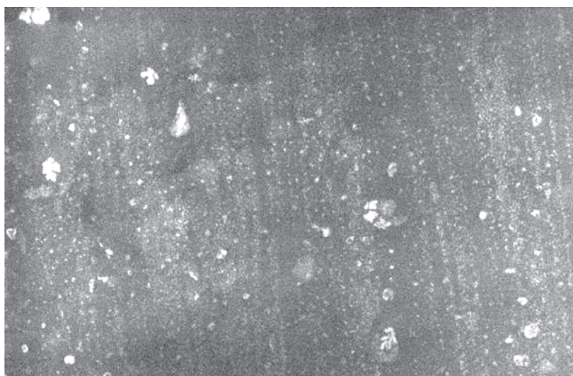
Fig. 2. SEM image of structure of TPE containing 10 pts. wt. of BS-100
