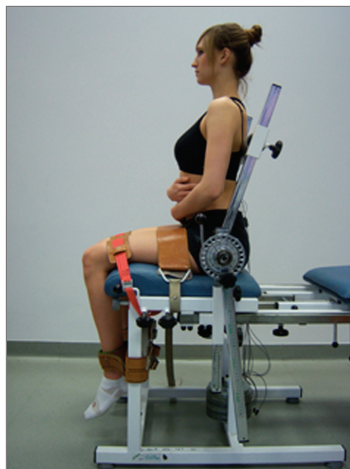
Fig. 2. Measurement of the maximum torque and EMG activity of back muscles
