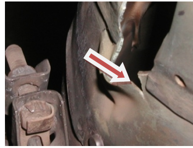
Fig. 5. Thermal damage of flame tube
