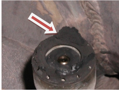
Fig. 4. Carbon deposits on injector
