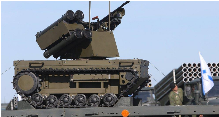
Fig. 1. A prototype of a heavy, autonomous combat platform Platform-M [Source: https://sputniknews.com/military/201507241025004070/ ]
