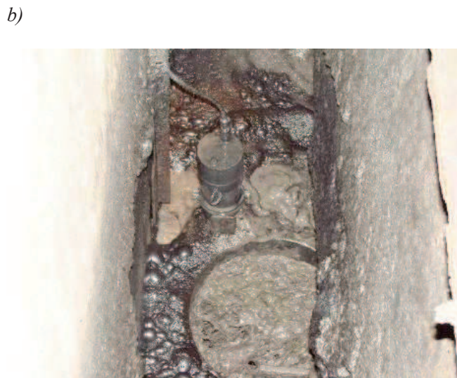
Fig. 14. MPOF2 Ash Meter: a) General view – basic elements: 1 - measuring head, 2 - visualization module, b) view of a built measuring head
