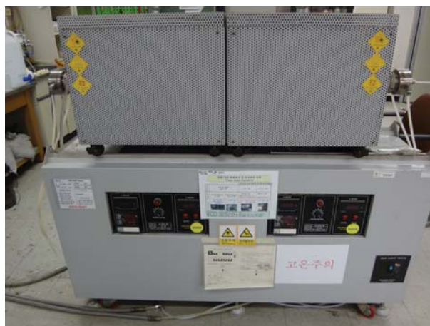
Fig. 1. Two-zone tube furnace.
