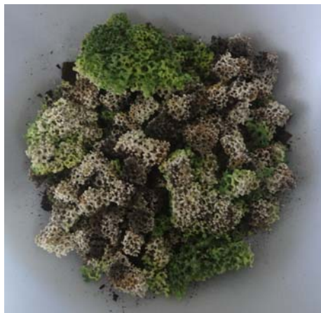
Fig. 7. The first granule filter of sponge structure (sample 5) after trapping.
