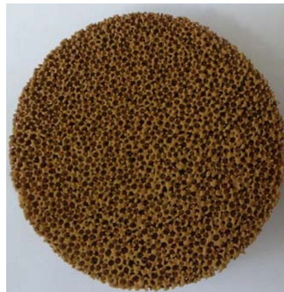
Fig. 4. Disk-type fly ash filter.
