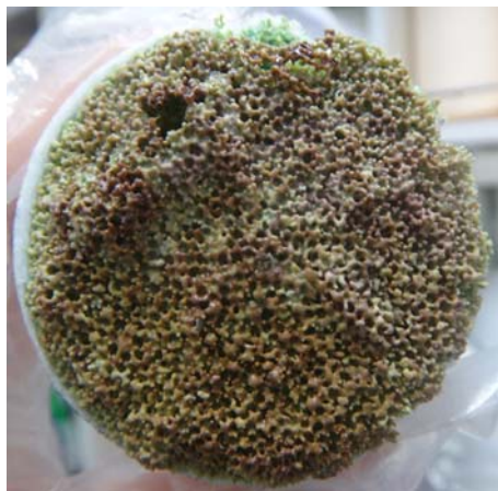
Fig. 6. The first disk-type filter after trapping.
