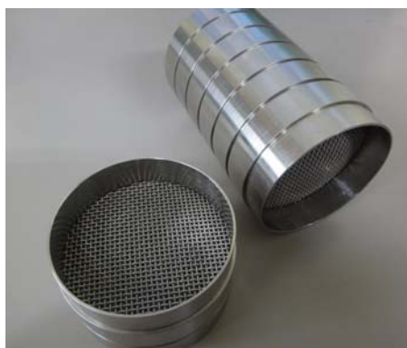
Fig. 2. Ring container for granule experiment.
