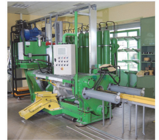
Fig.3. PH-LR 500 - a horizontal hydraulic press - 5 MN used for backward extrusion
