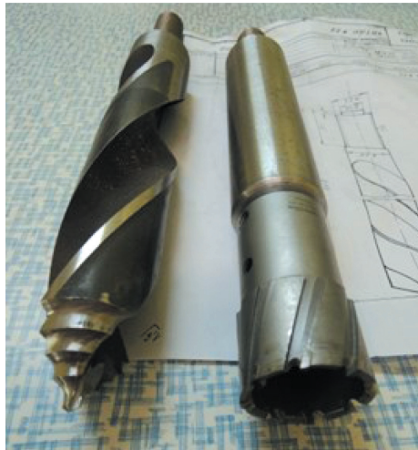
Fig. 9. Hot tapping device. Left: step reamer, right: magnetic bit
