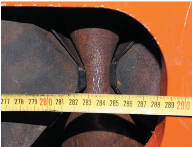
Fig. 4. Deformed 5" mud pipe in FIB-1 device while squashing with cone rams with welded additional elements
