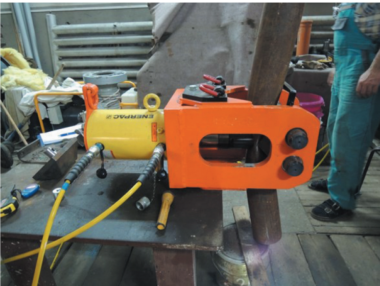
Fig. 3. FIB-1 during a 5" mud pipe squashing test
