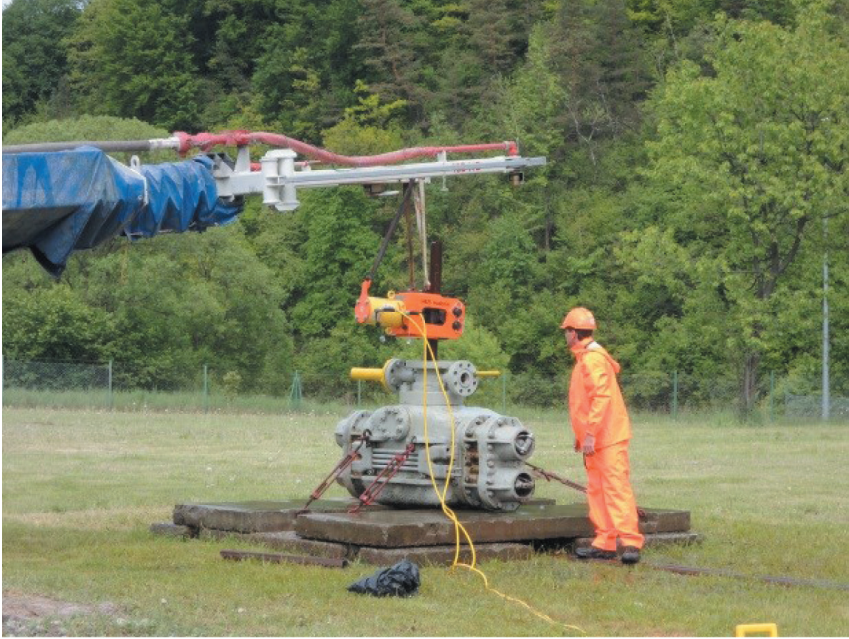
Fig. 6. Test of DPRP I device for reducing pipe blowout in an experimental zone of EXALO Drilling S.A. in Tarnawa Dolna, n. Sanok
