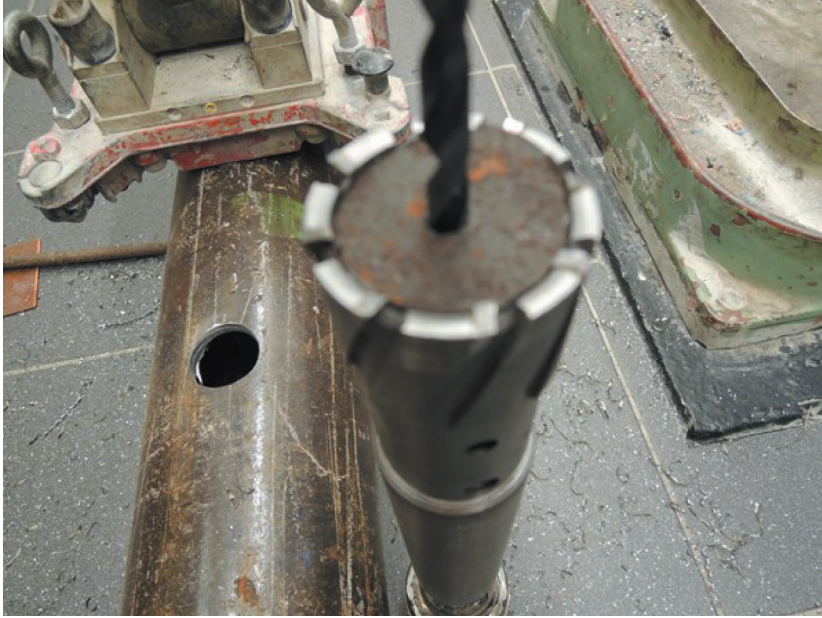
Fig. 10. View of modified bit with pilot drill. A hole in the casing in the background
