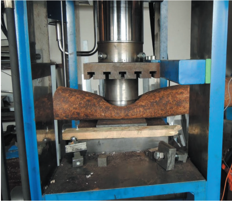
Fig. 2. Analyses focusing on the design of elastic pipe squashing press. SHREK HL-100T press with hemisphere/flat surface rams during the pipe squashing test
