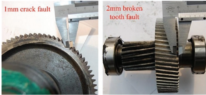
Fig. 5. Location of compound fault in gears
