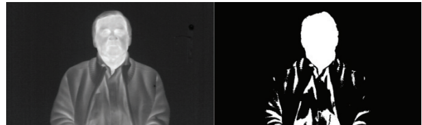
Fig. 1. Original thermographic and binary image after binarization using Otsu method [9]
