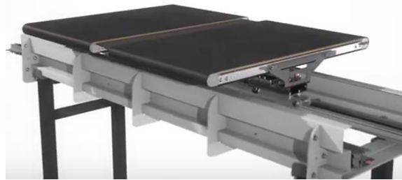
Fig. 2. Trays with transverse conveyors, placed on the trolleys directed in a track (enlargement of a detail from Fig. 1) [5]
