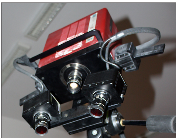
Fig. 8. ATOS I scanner used in the research
