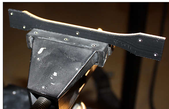
Fig. 9. Non-coded reference targets placed on measured object
