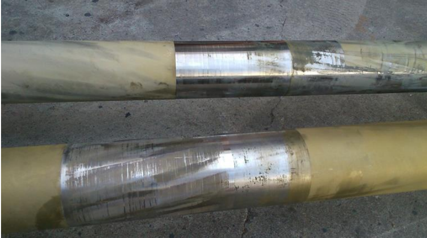
Fig. 5. Comparison of wear and tear shaftlines; visible signs of abrasion over the entire length of the spiral-rubber bearing resulting from the flexural buckling of the shaft shown at the top, the shaft shown in the bottom has the visible signs of proper lubrication contoured thread [author's photo]
