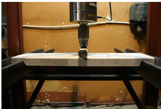
Fig. 11. Method of testing composite lining
