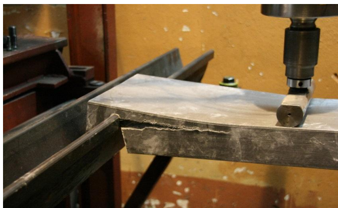
Fig. 21. Typical damage to a structural channel in the area of the V-profile's seat (sample 7)
