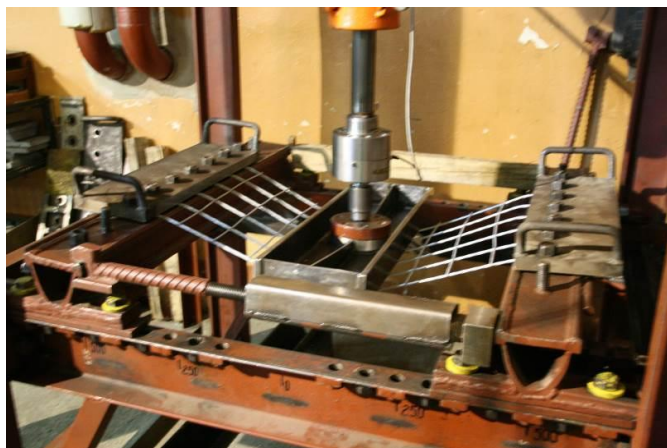
Fig. 10. Method of testing lining meshes
