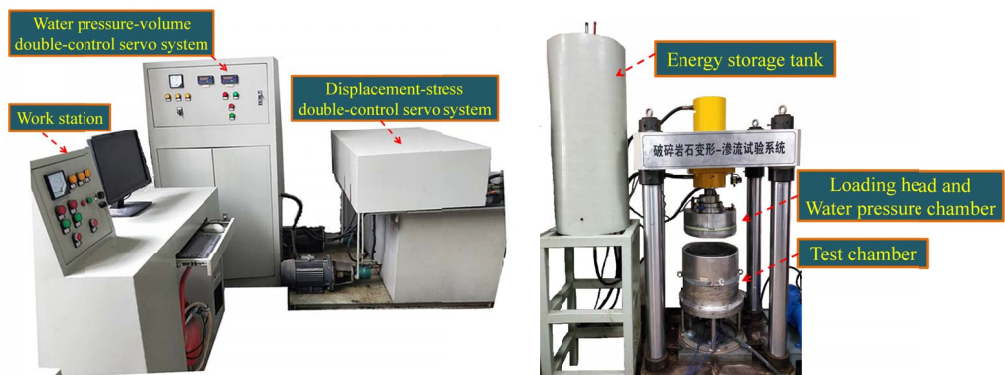
Fig. 2. Structure and system parameters of the crushed rock deformation-seepage test system
