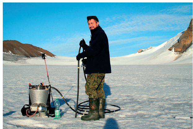
Fig. 1. Ice drilling with Heucke Ice Drill on glacier (photo M. Marciniak)
