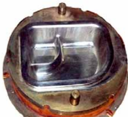
Fig. 2. The mould for a divided tray [21].
