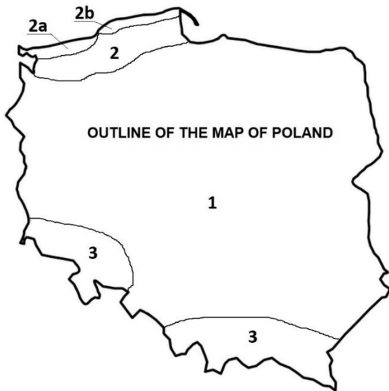
Fig. 8. Approximate division of Poland into zones of wind load according to PN-EN 1991-1-4:2008 [13]
