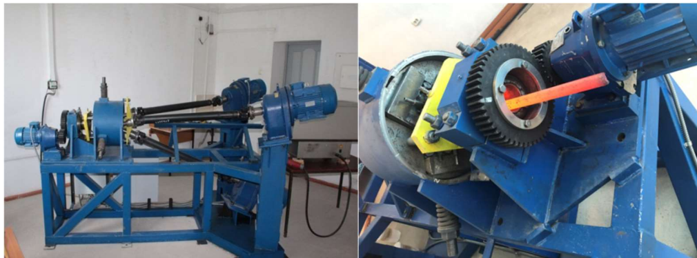
Fig. 3 Radial-shear rolling mill SVP-08 and rolling process on it
