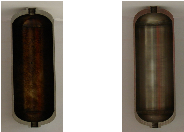
Fig. 6. Traditional non-dismountable sampler after a series of sample collection [left] and clean non-dismountable sampler [right]
