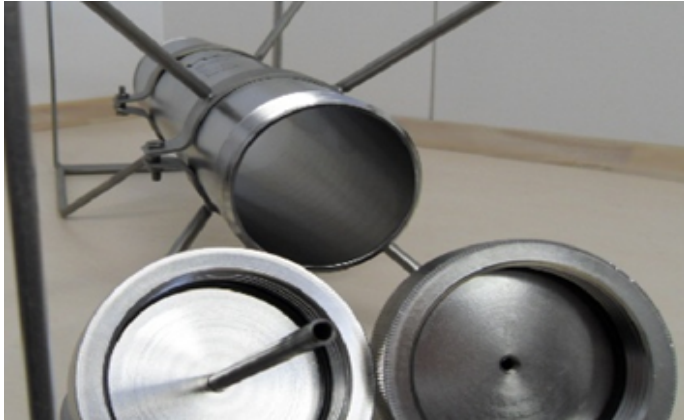
Fig. 5. Traditional non-dismountable sampler
