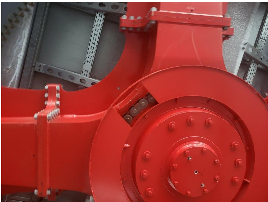
Fig. 9. Jawor station. Chain clutch-the ability to switch the main bearing to the emergency bearing [43]
