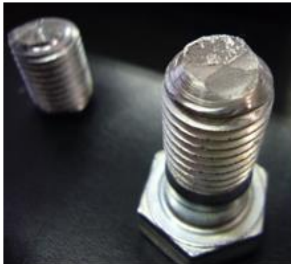
Fig. 5. Sheared screws of the emergency bearing ring [6]
