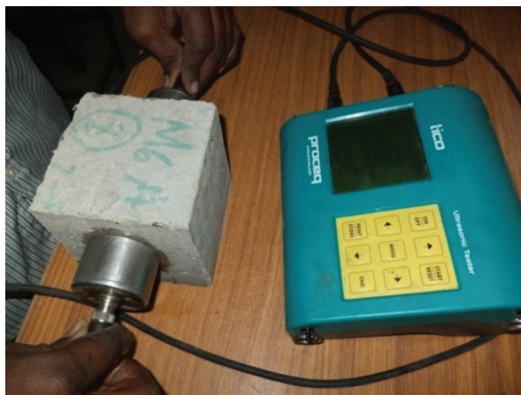
Fig. 4. Test set up for Ultrasonic Pulse Velocity
