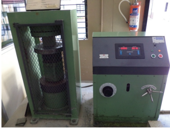
Fig. 3. Test set up for Compression testing machine
