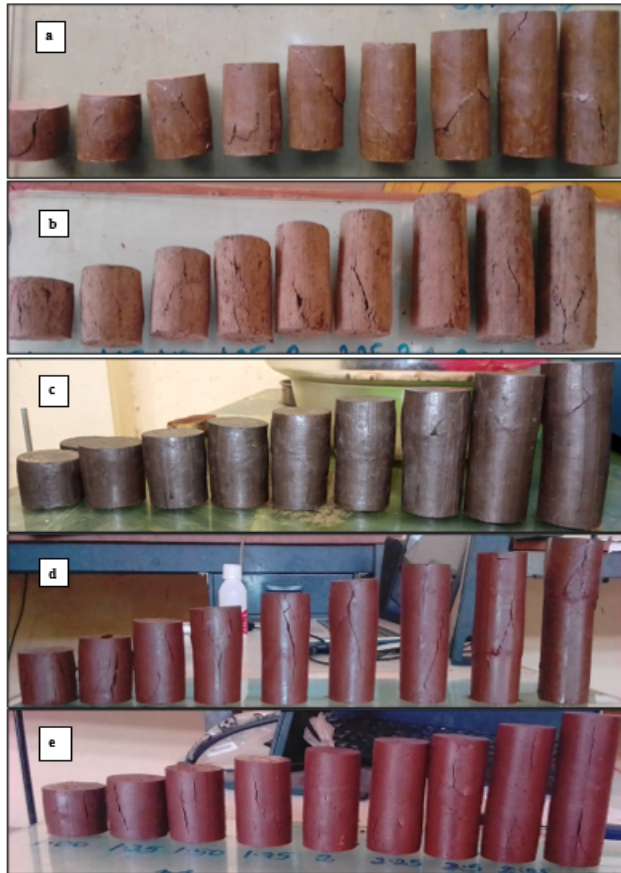
Figure 9: Failure pattern of 38 mm specimen diameter: (a) Ajip, (b) Aweyту, (c) JIT campus, (d) Saris Sefer, and (e) Mariam Church.
