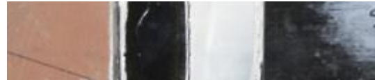
Fig. 4. The CFRP-HARDOX specimen tested at RT, the adhesive failure (adhesive remains on one adherent)
