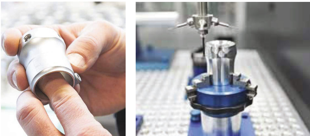
Fig. 4. Each component of a prosthetic must meet the design requirements exactly. The measuring machines must also correctly display complex geometries
