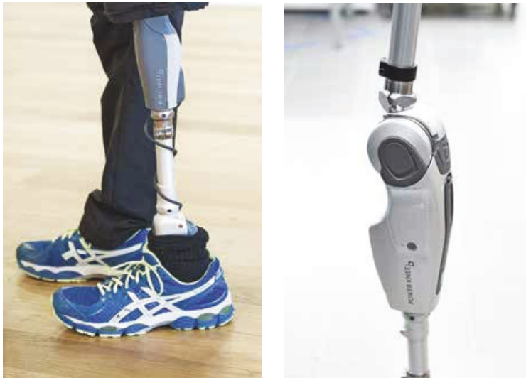
Fig. 2. A prosthetic leg must be able to bear the weight of the user nearly one million times a year. The Power Knee high-tech prosthetic can replace the muscle activity of people whose legs were amputated above the knee
