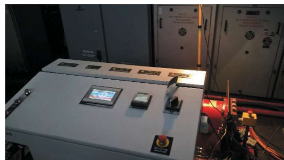
Fig. 7. Measuring system for validation tests of the electric drive in the riding and operation mode
